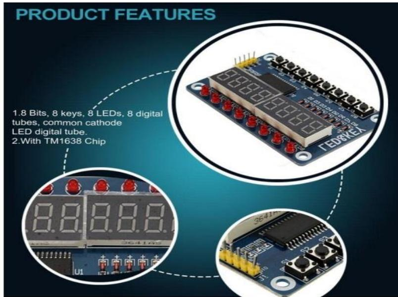
The board has 3 control pins plus power and ground.
